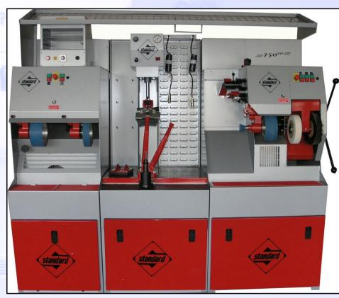
The Standard 625mm Pressbench as part of our "Mini" and "Maxi" Repair Units
