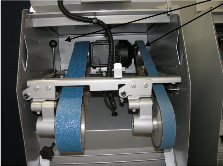
Band Tension Release Levers
