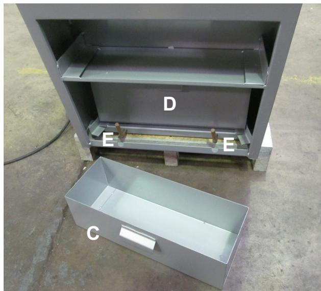
To remove the waste levers (E) by moving
