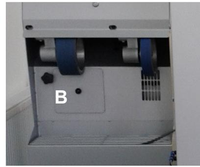
**The Dust Collection Trays** are situated behind the access door in the base of the machine. THESE MUST BE EMPTIED DAILY OR REPEATEDLY DURING THE DAY IF MACHINE IN CONSTANT USE.
