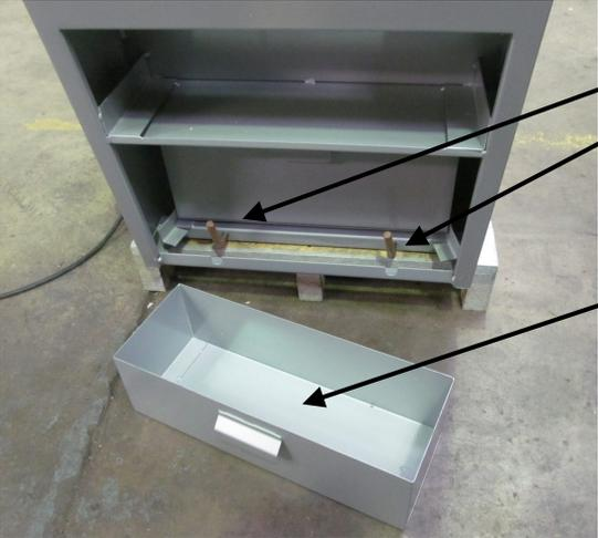
Dust drawer sealing levers. Drawer is sealed when levers are vertical
