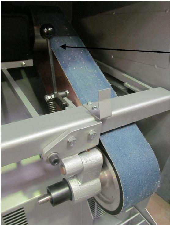
Band Tension Release Lever
